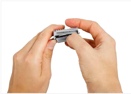
Open the Gelbox at the side latches.
