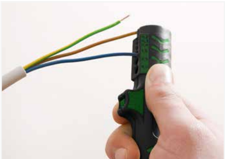
Stripping a conductor insulation.
